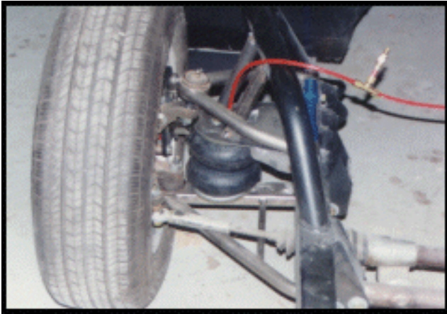
Aftermarket Mustang II installation [replaces coilover shock]
