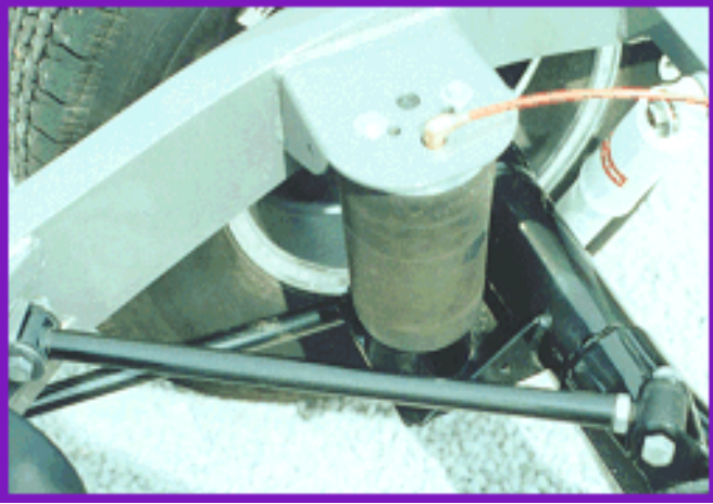
Rear suspension w/ 4 link and air ride
