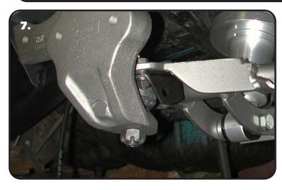
**7.** Attach the Spindle to the control arms.
