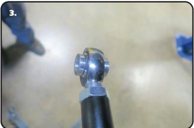
**3.** Install the ¾" jam nut onto the end of the Heim end, then screw Heim end into the end of the panhard bar. Set the Panhard Bar to 31.500". You may need to readjust it after getting the car set at ride height, but this is a good starting point. Press the SMALL diameter of the aluminum 9/16" ID T-bushings into the Heim end.
