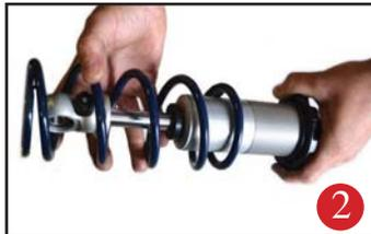
2 Next install delrin washers then coil spring over the top of the shock as seen in figure 2
