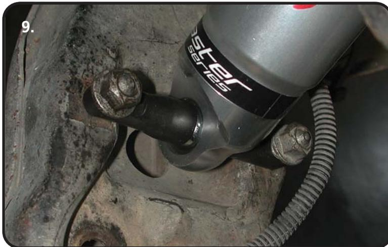
9. Attach the lower CoilOver mount to the OEM Lower Control Arm using (2) 3/8"-16 x 3" Bolts, (4) 3/8" Flatwashers, and (2) 3/8"-16 Nylok Nuts. Tighten Hardware. It may be necessary to raise the lower control arm up to align the CoilOver with the OEM Mount.
