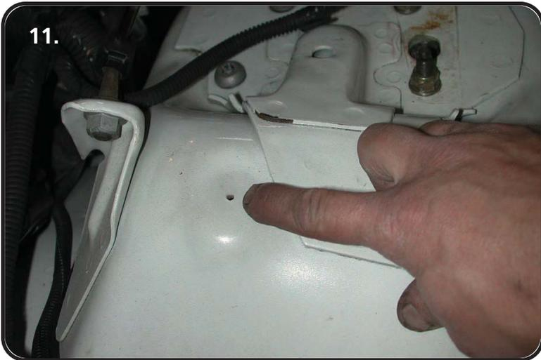
**11.** A bump stop will be installed between the inner fender and upper control arm to ensure that the tire does not hit the inner fender when fully compressed. There is a small hole on the inner fender that must be drilled out to 3/8". Fasten the bump stop to the inner fender using a 3/8" Nylok nut and flat washer.
