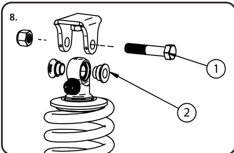
**8.** Install the 1/2" I.D. Spacers (1) into the bearing of the upper CoilOver eyelet. Insert the CoilOver into the upper mounting bracket aligning the holes in the spacers with the holes in the bracket. Insert 1/2" x 2 1/2" bolt through the bracket and CoilOver. Install 1/2" Nylok nut and tighten.
