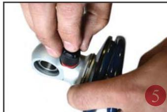
5 Install upper spring mount retainer clip (90002057) into the groove on the upper eyelet as seen in figure 5. Then reinstall adjuster to complete assembly.
