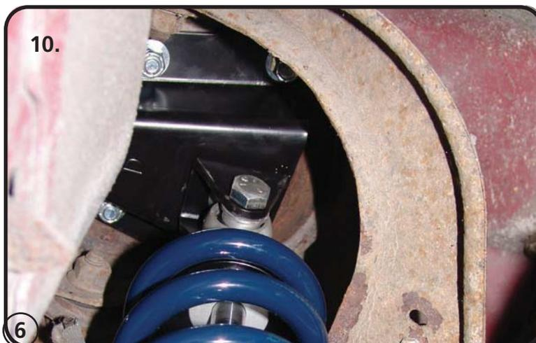
Tighten the lower Coilspring Adjusting nut until the Coilspring is sitting snugly on the CoilOver. Using the Spanner wrench add another 1/2" of preload in the spring by threading the adjuster nut up the Shock Body. Be sure that the locking screw is lightly tightened in the adjuster nut. Once you have preloaded tighten the locking screw. It may be necessary to add more preload, this will be determined once the car is setting on the ground.
