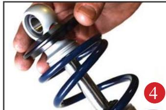
4 Slide the Derlin washer over the spring, Next slide the upper spring mount (90002222) over eyelet as seen in figure 4.
