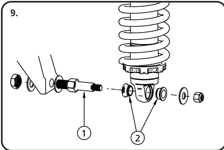
9. Drill the factory shock stud hole out to 5/8" , this can be done using a Unibit. Install the (1) Shock stud (90001617) into the factory lower mount using the hardware supplied with the stud. Install a 5/8" I.D. spacer on the shock stud, then the bottom of the ShockWave on the stud, followed by another 5/8" I.D. spacer. Install 7/16" washer and Nylok nut.
