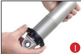
1 First using the supplied lower adjuster nut(90002222) thread the nut onto the shock from the top side as seen in figure 1
