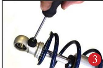
3 Before the upper spring mount can be installed screw the adjuster knob on the upper eye mount to the firmest setting (clockwise) as seen in figure 3. and remove knob.
