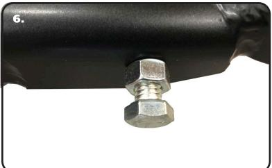
**6.** Thread the 3/8"-16 nut onto the 3/8"-16 x 1 ¼" bolt. Thread it into the front hole of the ball joint plate. You will need to adjust the steering stop to suite your needs. This setting will vary depending on wheel and tire size and other suspension components. Torque to 12 ft-lbs.
