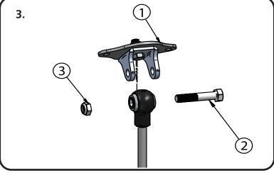
3. With the upper mount installed insert the Shock assembly into the upper shock mount(1). Align the holes in the bracket with the hole in the Shock sleeve and insert the 1/2" Bolt(2). With the Bolt insert install a 1/2" Nylok Nut(3) and tighten.
