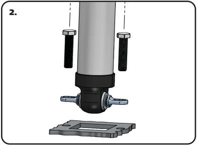
**2.** Attach the Trunnion to the OEM Control arm using the OEM hardware. It made be necessary to rotate the Trunnion to get it in the correct position. This can be done by sticking a screwdriver in one of the slots and spinning the trunnion in the shock bushing.
