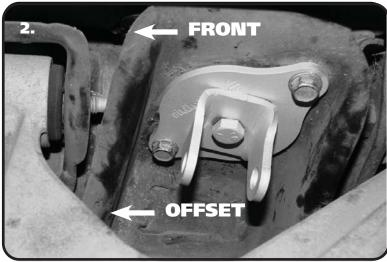
**2.** Install the upper mount into the car using the factory hardware. The Mount will have the top of the Shock OFFSET TO THE FRONT OF THE CAR.
