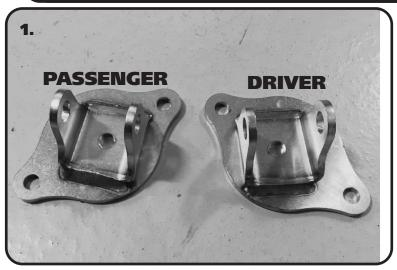
1. Start be removing the OEM shock. With the shock removed start installing the New HQ Series shocks. The Upper Mount will be replaced with mounts included in the Shock Kit. The new Upper Mounts will offset the Shock to the front of the Corvette. When these mounts are installed correctly, the Upper Mounting Bolt will be PARALLEL with the Lower Mounting Bolt.
