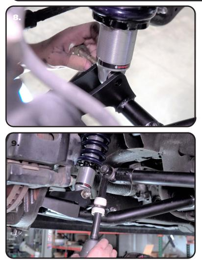
**8.** Install the 1/2" I.D. bearing spacers into bearing in the shock body. These spacers have a through hole that is 1/2" diameter. The small end of the spacers will insert into the shock bearing. Slide the shock with the spacers installed into the lower control arm. Raise the arm up to line up the holes in the bushing with the 1/2" hole in the control arm straps and hold it in place. You may want to put a jack under the lower control arm to help hold the control arm in position.
