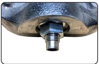
**5.** Reinstall the OEM washers and nuts on the lower control arm bolts. Torque to 129 ftlbs.
