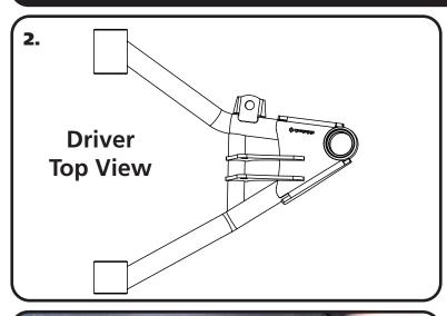
**2.** The lower control arm is attached to the factory mounts using factory hardware. The driver side arm is shown in **Figure "2"**. The sway bar tab on the control arm will be to the REAR of the control arm.
