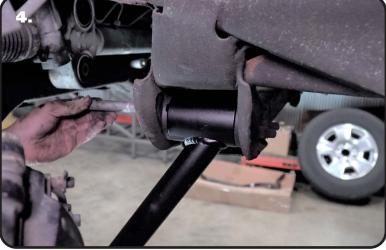
**4.** With the bushing sleeves aligned with the OEM mounting holes, reinstall the OEM control arm bolts.
