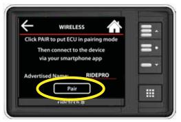
**Step 2:** Go to the Wireless tab under the Menu on the control panel and select it. You should see the screen above. Touch the pair button on the control panel.
