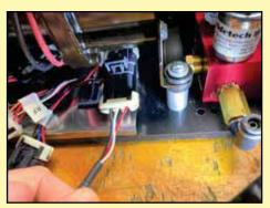
**AIRPOD ONLY!** Start the plug on the retainer and slid it until it clicks. This will lock the harness in place.
