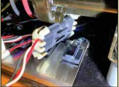
**AIRPOD ONLY!** The AirPod has 4 clips on the main board to secure the plugs for the level sensor harnesses. The female plug on the sensor harness will attach to these clips. The plug slides onto the clip from the release side of the clip.
