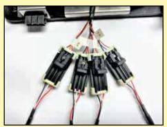
Run the harness from the sensors to the Main Harness (AirPod). We recommend marking the harnesses at the end that will plug in at the Main Harness (AirPod). The 4 plugs in the Main Harness are labelled for each corner. Plug the correct harness into each plug.
