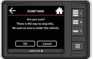
Dump Tank has a secondary screen to verify you want to dump the tank.
