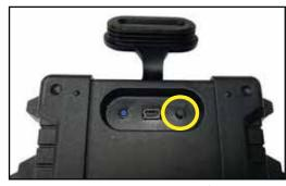
**Step 2:** Open the rubber cover on top of the ECU. Push the button that is under the rubber cover. The Blue light will start flashing.
