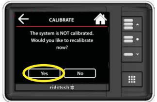
Make sure nothing is under the vehicle before performing calibration. To Calibrate the system, select "Yes".
