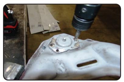
**1.** If your Ball Joints are Bolted to the Control Arms, simply unbolt them. If your car has the Original Ball Joints, they will be Riveted to the Control Arms. The Rivets can be removed by Grinding the Heads off and driving the out with a Hammer and Punch.
