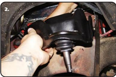
2. Insert the Ball Joint into the Control Arm from the top side of the Control Arm with the Ball Joint Pin Sticking down. Attach it to the Control Arm with the Hardware Supplied with the Ball Joint. Torque the Hardware to 14 ftlbs. Engage the Ball Joint Pin into the Spindle and install the Castle Nut Supplied. Torque the Castle Nut to 50 ftlbs and tighten to align Cotter Pin Hole. Install Cotter Pin through Hole and Bend Pins to prevent falling out.
