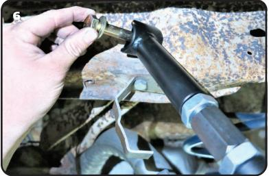
**6.** Remove one of the upper bar bolts. Install a 1/2" SAE flat washer on a 1/2"-20 x 4 1/2" bolt. Align the top of the frame brace with the top upper bar hole. With them aligned, insert the bolt/washer in the aligned holes. Install a 1/2" SAE flat washer and 1/2"-20 nylok nut on the threads of the bolt. Snug down the hardware, but leave it loose enough to move the brace for alignment of the lower bolt.
