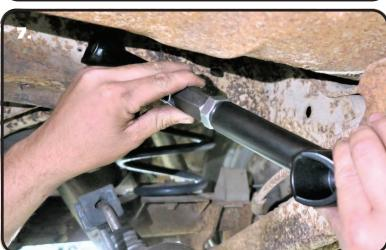
**7.** Remove the OEM bolt out of the front lower control arm. Position the bottom mount of the brace close to the lower control arm mounting hole. While holding the bottom of the brace in position, turn the adjuster until the bottom brace hole is aligned with the lower control arm hole.
